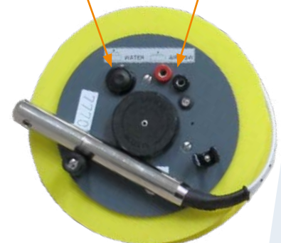
Water or air switch Cable connections
